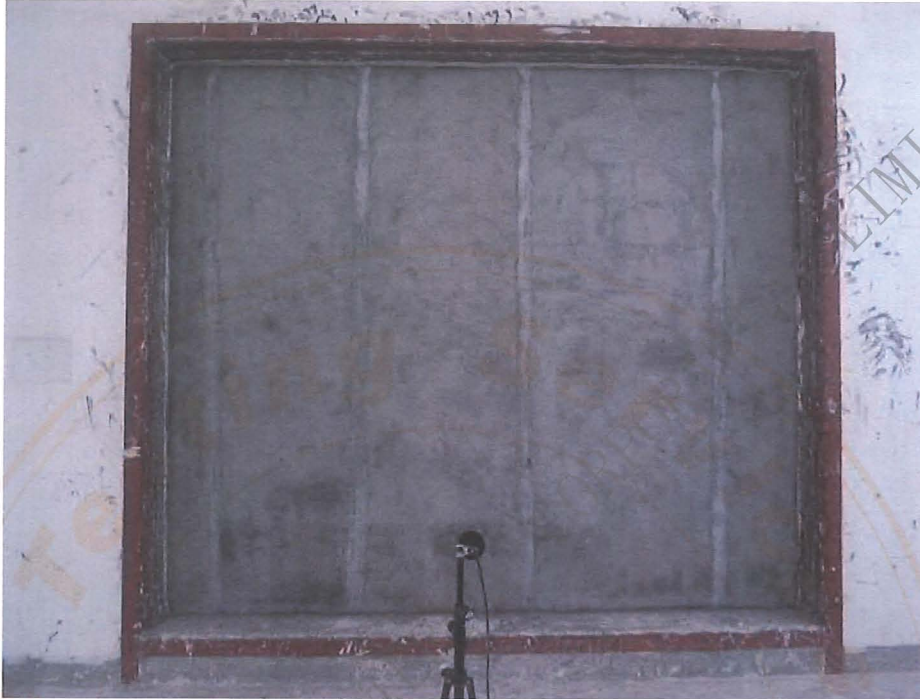
Set-up of Unit Under Test (Source room)
