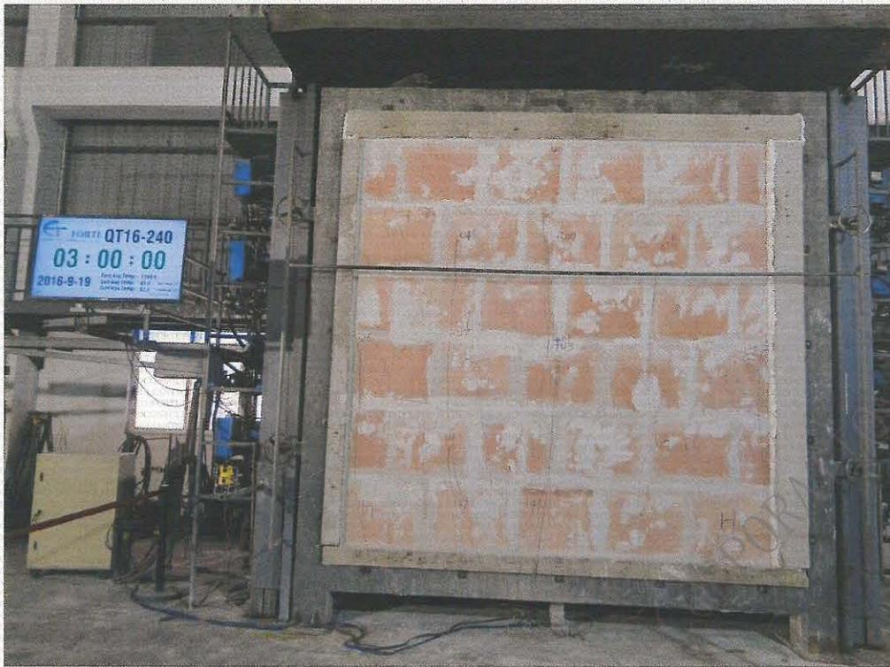
**Photo 9.** Unexposed surface of the specimen at 180 minutes of test.
