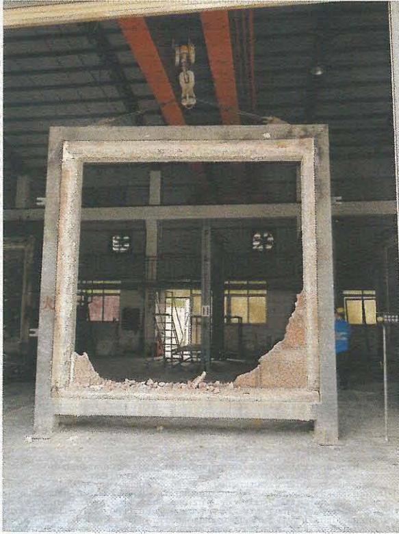
**Photo 13.** Fire exposed side of a portion of the specimen on the test rig after the test.
