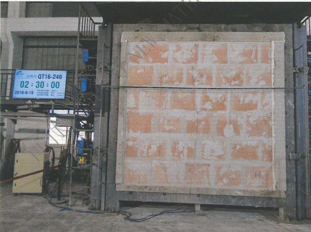
**Photo 8.** Unexposed surface of the specimen at 150 minutes of test.
