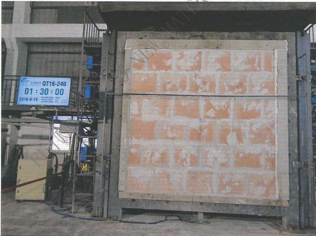
**Photo 6.** Unexposed surface of the specimen at 90 minutes of test.
