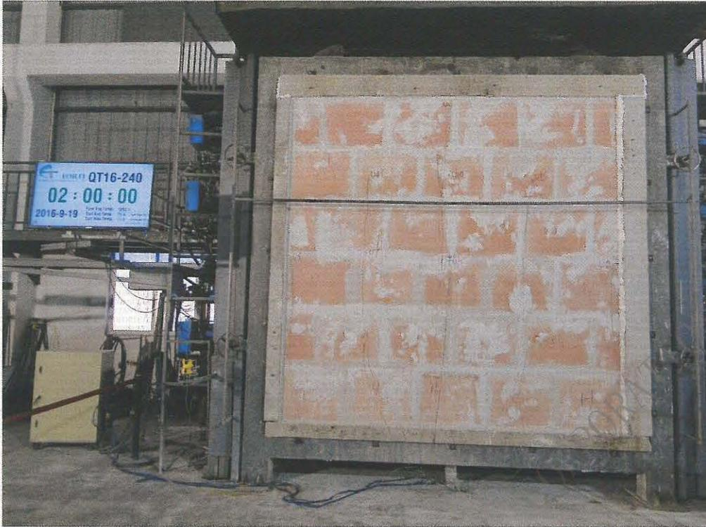
**Photo 7.** Unexposed surface of the specimen at 120 minutes of test.
