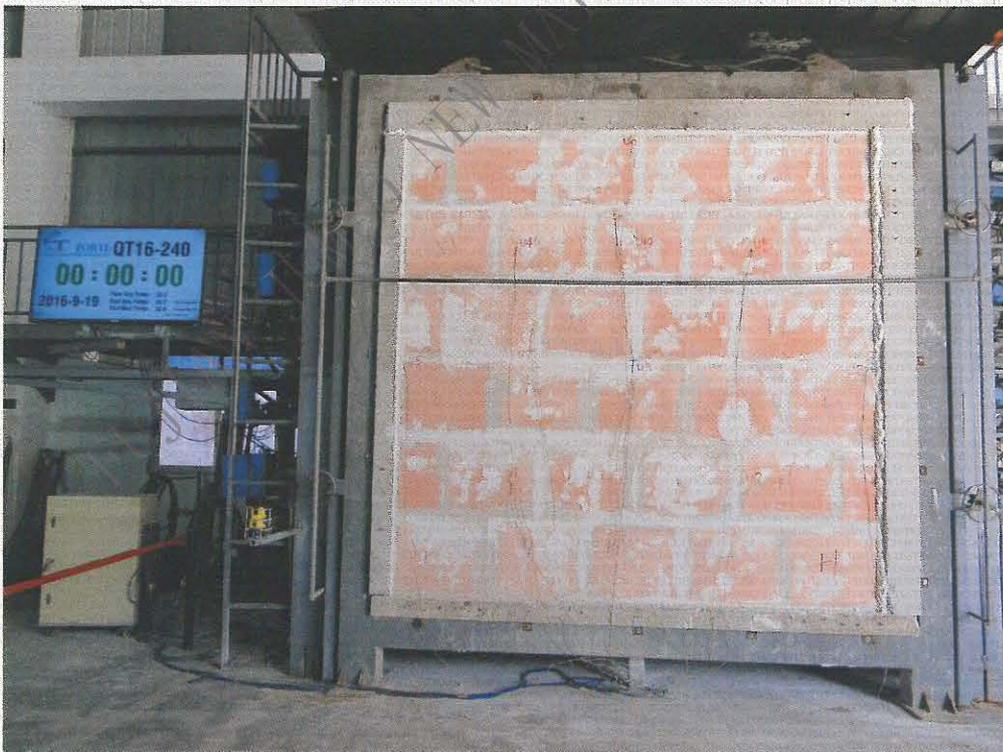
**Photo 2.** Unexposed surface of the specimen before the commencement of test.
