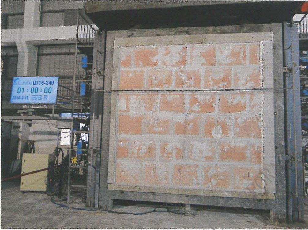
**Photo 5.** Unexposed surface of the specimen at 60 minutes of test.
